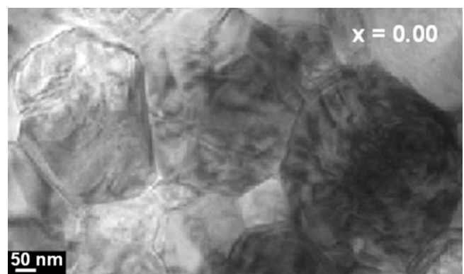
Fig. 9. Bright field TEM images of \text{Ba}_{1-x}\text{La}_x\text{TiO}_{3-\delta} ceramic samples (obtained at 1050 °C) showing grains with sizes of 600 nm which correspond to the D_{\max} value determined among all compositions.
